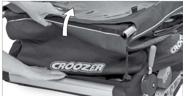
3. Holding the upper frame tube in the raised position, pull the seat frame slowly and carefully back and towards you until the locking pins (5) of both locking mechanisms (4) engage with audible clicks in the holes (6) of the frame tubes.
