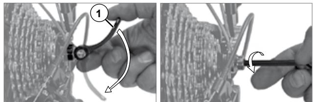
The quick-release lever must be positioned on the right side of the bicycle (relative to the direction of travel). If the lever is on the left side, the quick-release skewer must be removed and reinserted from the right side. Be sure to follow the applicable instructions in the owner's manual of the bicycle and/or consult a professional bicycle mechanic.
