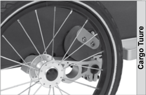
Maintenance-free AirPad® suspension with Sylomer® (Cargo Tuure)
