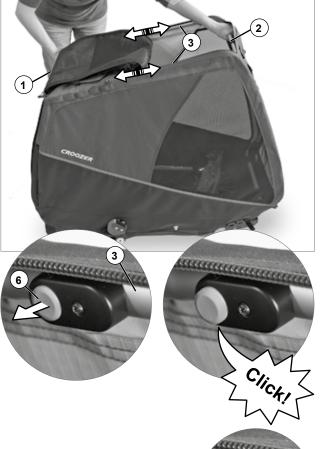
7. To fold the Croozer, follow these instructions in the reverse order. Press the buttons (6) of the locking mechanisms on both sides, and push the sections of the frame together. (See page 32 for a more detailed description.)
