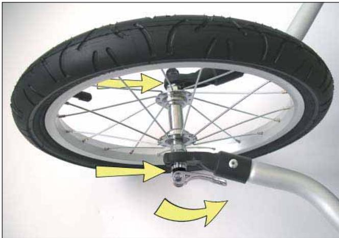
If the jogger wheel cannot be pushed into the dropouts, undo the adjusting nut of the quick-release, turning it anti-clockwise.
