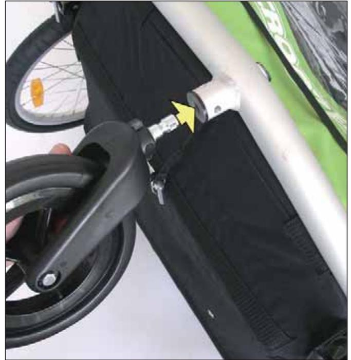
Insert the security pin through the hole in the bush.
