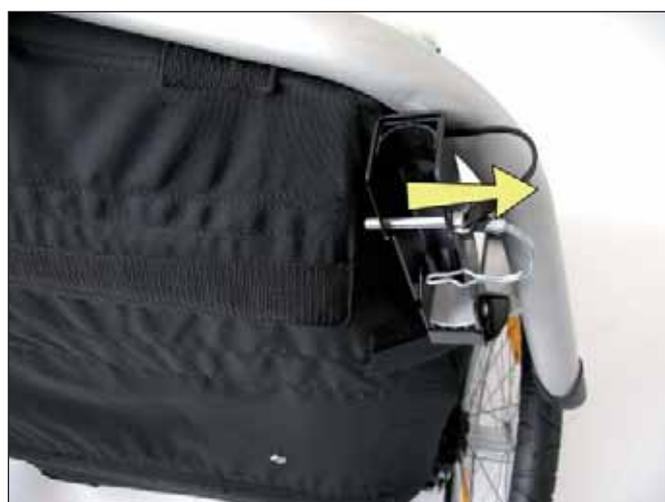
The hitcharm should be attached to the Carrier so that the hole at its rear end is facing upwards.
