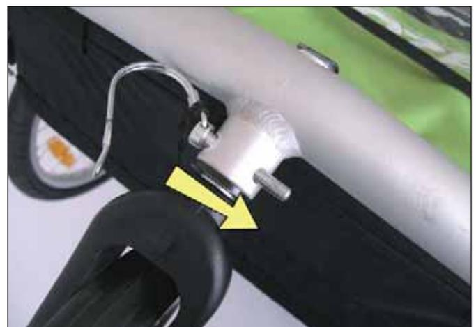
Secure the security pin in position by letting the safety clip snap over the pin.
