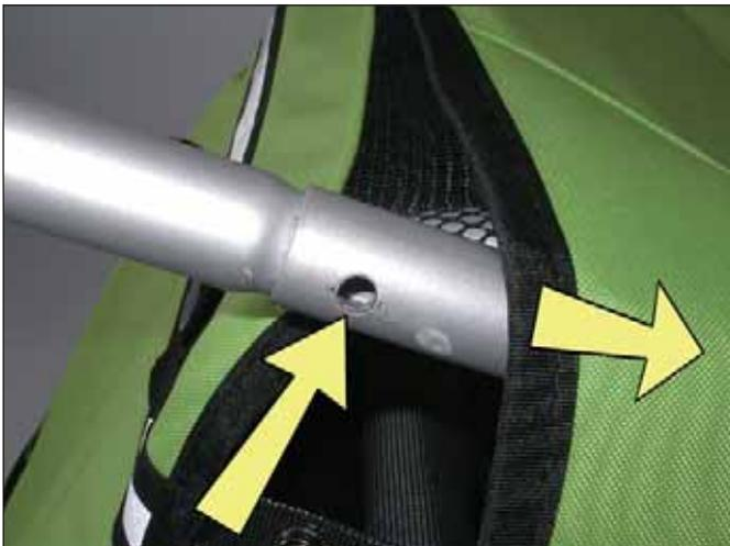
Engage the handlebar in position by inserting the two security pins through the aligned holes in the handlebar and frame tube as described. Secure the security pin in position by letting the safety clip snap over the pin.
