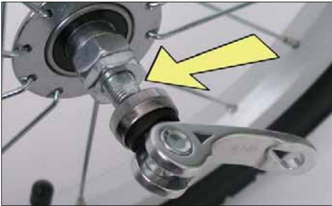
Open the quick-release lever of the jogger wheel as far as possible. Push the jogger wheel into the dropouts of the wheel arms so that the flat points of the axle are parallel to the slot in the dropouts.
