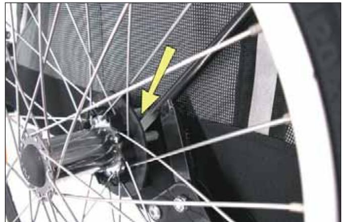
To release the brake, press the lever downwards as far as it will go.
