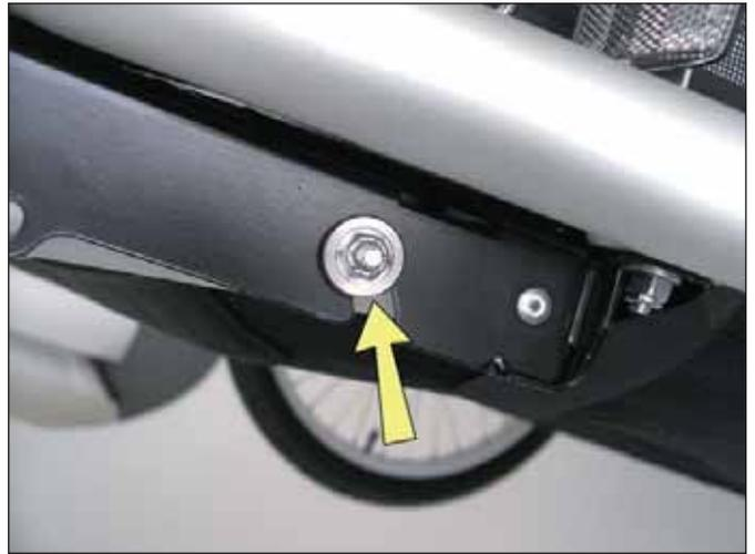
Insert the rear end of the hitcharm into the rear end of the hitcharm attachment bracket.
