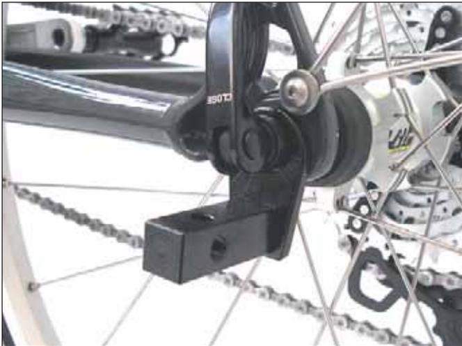
The quick-release is properly adjusted when you can clearly feel resistance as you are about to fully close it. You should feel this resistance about 60° before the end of the lever movement. If it is too easy or too difficult to move the quick-release lever, slightly tighten or loosen the Q.R. lock nut on the other side of the hub.
