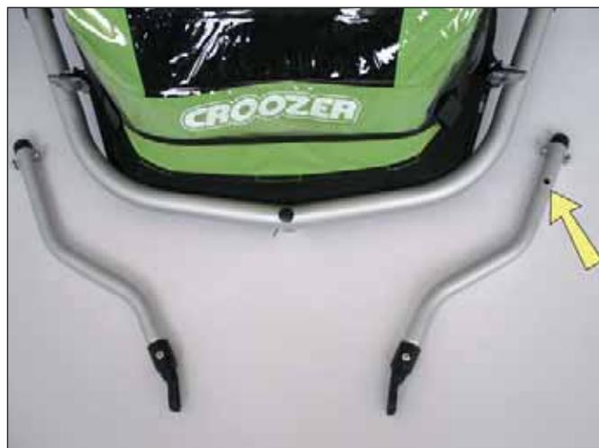
The two wheel arms are fitted and secured in the same way as insertion of the hitcharm (see Section 5.5).
