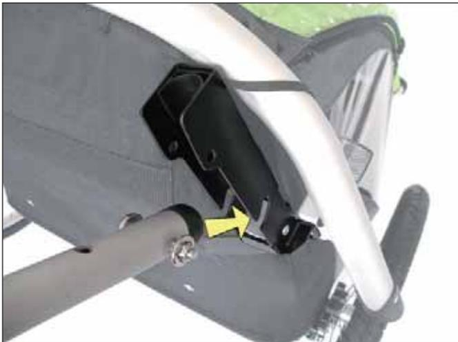
The bolts on the sides must engage in the slots of the attachment bracket.
