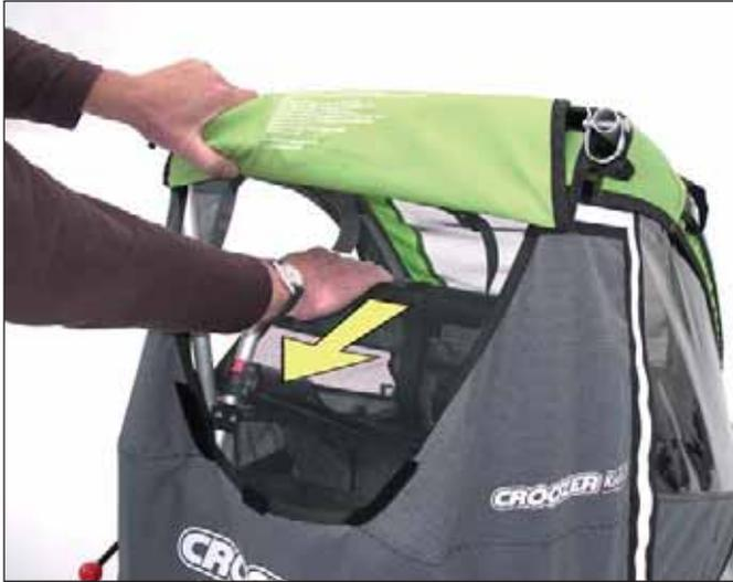
Now close the left Auto-lock disk in the direction of travel. The left Auto-lock disk is properly closed once the red catch has snapped into place over the frame tube that points upwards.
