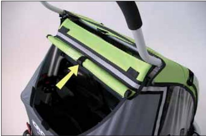
The snap fasteners on the Carrier are each attached to a loop. To make it easier when it comes to refastening the snap fasteners, slide a finger under the loop.
