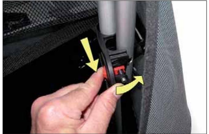
Let go of the red sliding button. The locking pin should now click into its designated hole in the frame tube that points upwards. To achieve this, once you have let go of the sliding button, you might have to move the Auto-lock disk backwards and forwards slightly.
