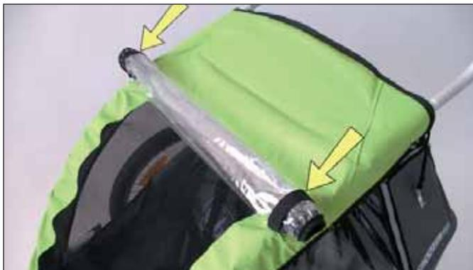
The entire two-in-one weather cover can also be rolled up and held in place by means of a strap in the centre. For this, the transparent window must be rolled down and attached in place to its fabric surround.
