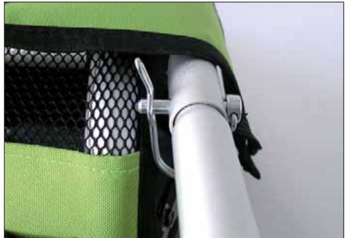
Pull the rear end of the two-in-one weather cover back over the security pin again. Make sure the snap fasteners that hold the two-in-one cover in place are closed (see Section 4.4).
