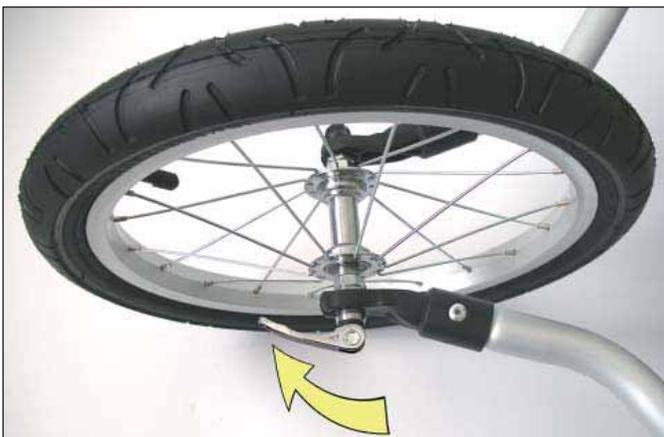
The quick-release is properly adjusted when you can clearly feel resistance as you are about to fully close it. You should feel this resistance about 60° before the end position of the quick-release lever.
