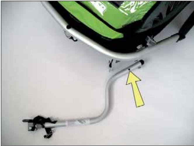
Press the hitcharm upwards so that the bolts slide upwards into the slots.
