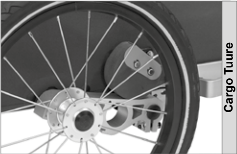
Maintenance-free AirPad® suspension with Sylomer® (Cargo Tuure)
